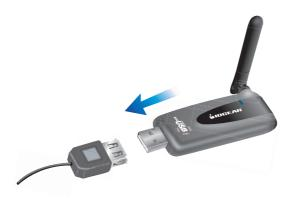
Place the extension cable on a flat surface, preferably the top of the desk/work area in order to ensure a good line-of-sight signal with the Wireless USB Hub. Windows should detect the device and complete the driver installation process automatically.
